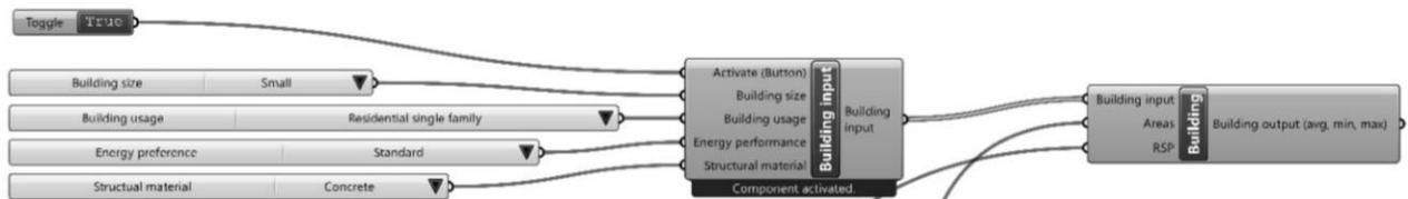
**Figure 25:** Simplified input on building level using the four categories as drop-down selections. SFH = single-family house; MFH = multi-family house
