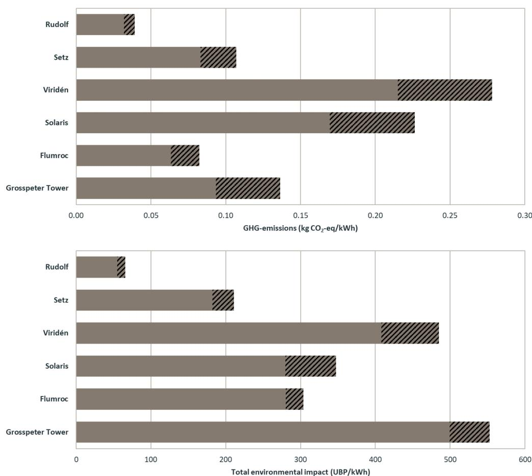
**Figure 5:** Gross greenhouse gas emissions (in kg CO<sub>2</sub>-eq, top) and gross environmental impacts (in eco-points, bottom, see also case study 1.3D3-01) per kWh electricity produced by the active glass façades of six BIPV buildings. The shaded area can be attributed to the building (impacts of front glass and supporting structure) and not the electricity production.
