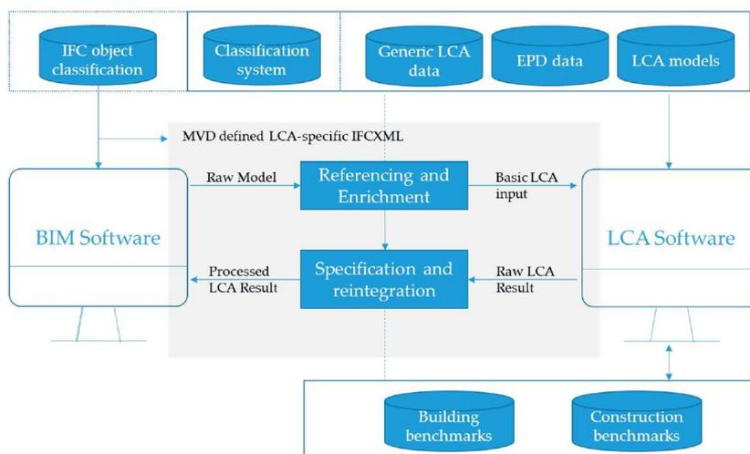
**Figure 39:** General workflow of the BIM2LCA approach as an extension of the strategies defined by <sup>[1]</sup> IFC-based bidirectional BIM-LCA integration.
