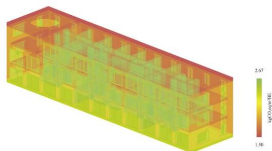
Fig. 7. Difference between average and optimal solution for each building element; expressed per  $m_{GFA}^2$ .
