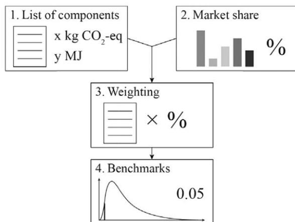
**Figure 16:** Simplified input on building level using the four categories as drop-down selections
