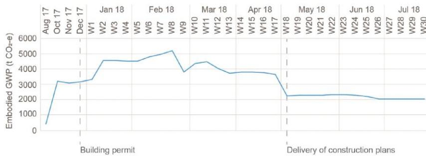
**Figure 48:** Evolution of total results for embodied GWP in t CO<sub>2</sub>-e throughout the design process.
