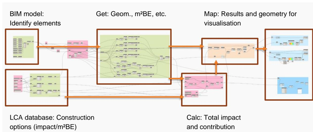
Figure 43: Custom script using a Revit BIM model and Dynamo for visual programming.
