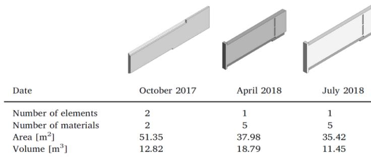
**Figure 49:** Example for quantity take-off for a single wall.
