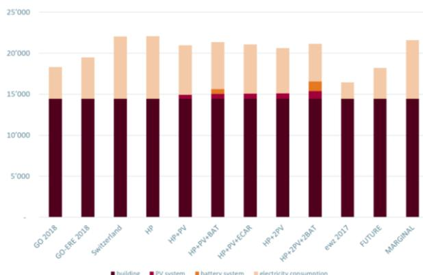
**Figure 2:** Environmental impacts (in Swiss eco-points 2013, see case study 1.3D3-01 from original publication) per m<sup>2</sup> and year of construction (building, PV system and battery, including end of life) and operation (electricity consumption) of the residential building Rautistrasse, Zürich, CH.
