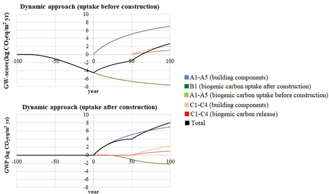
**Figure 10:** Global warming (GW) scores of the analyzed building as a function of the reference service life (year 0 is the construction of the building).
