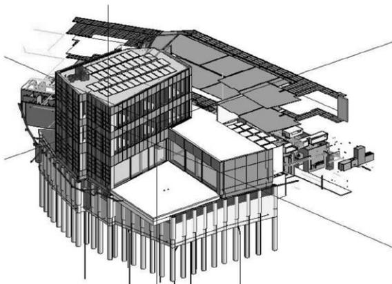
Figure 46: Example BIM model for the case study – the first office building in Switzerland built without printed plans
