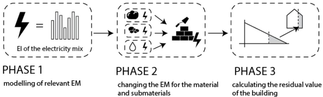
**Figure 7:** Three-phase approach to re-modelling the existing datasets and calculating the residual value of a building with the time-corresponding electricity mixes
