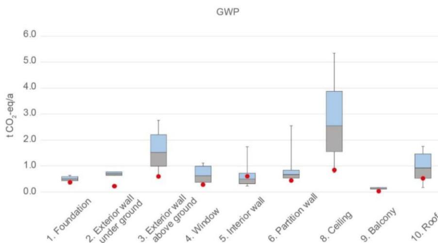
Figure 19: Benchmarks for the individual elements considering the surface areas of the building (points indicate the value for the specific material chosen in the case study)
