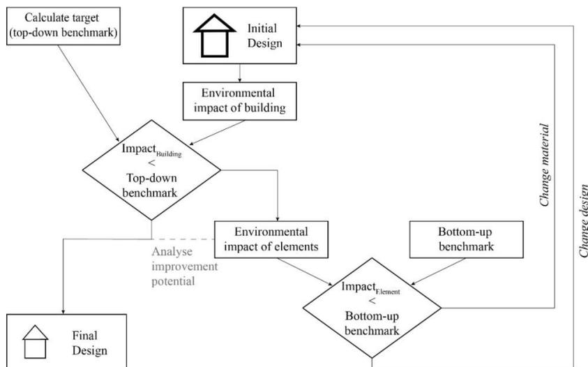
**Figure 17:** Proposed method of using the benchmarks in the design process
