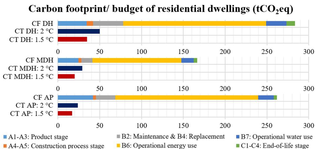
**Figure 15:** Carbon footprint and carbon budget of the New Zealand new-built residential dwellings over a 90-year estimated service life. CF= carbon footprint; CT= climate target; DH= detached house; MDH= medium density house; AP= apartment.
