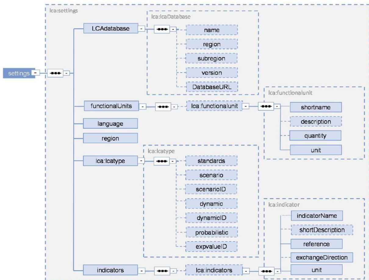
Figure 40: Example for LCA settings in the structure of a life cycle element.
