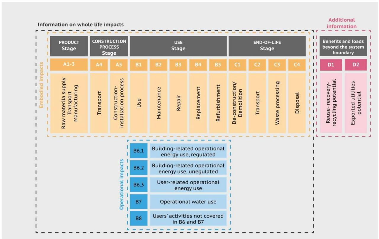
**Figure 1:** Display of modular information for the different stages of the building assessment as adapted from EN 15643:2021.
