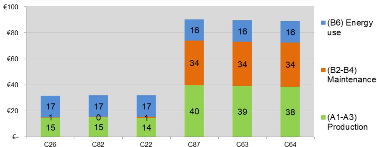
Figure 6: NPV of the total environmental cost of the three flat roof alternatives with best and worst performance (6 alternatives) within the total of the 114 alternatives assessed.
