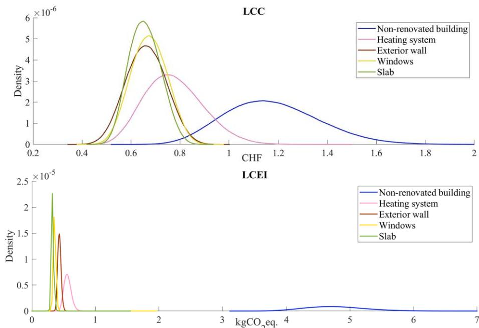
Figure 23: Measures applied following each iteration of the sensitivity analysis. The top graph shows results of uncertainty quantification for LCC in total CHF (Swiss Franc). The lower graph shows results of uncertainty quantification for LCEI (Life Cycle Environmental Impact) in total  $\text{kg CO}_2\text{eq}$ .
