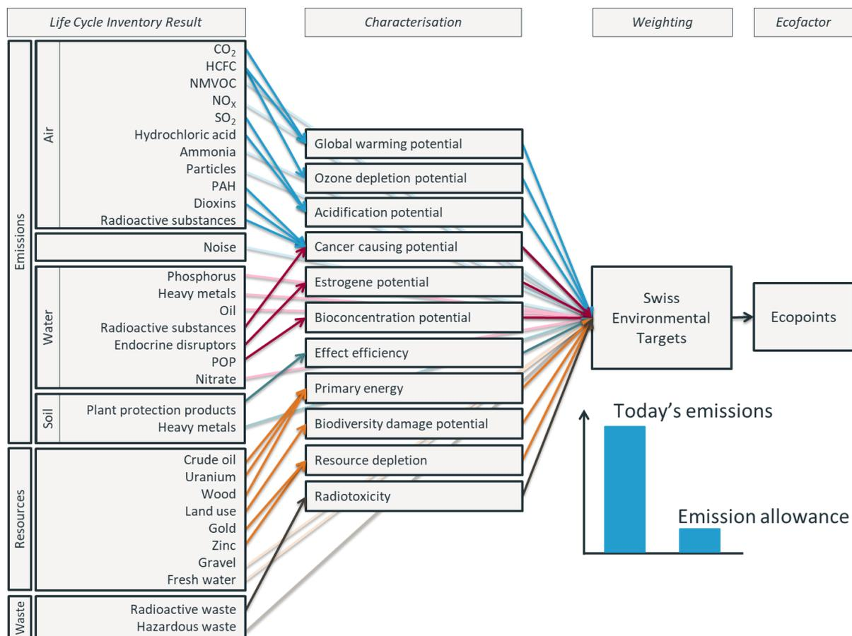
**Figure 12:** Basic concept of the ecological scarcity method, used to derive the Swiss eco-factors 2013.
