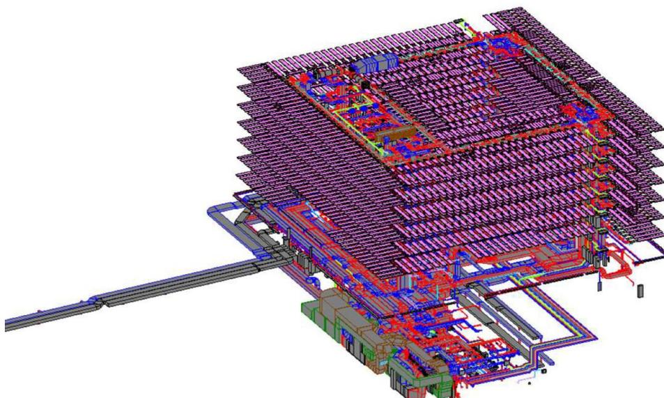
**Figure 33:** The BIM model of the HVAC systems of the case study building
